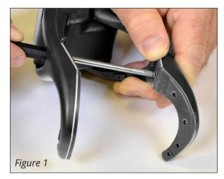
Completely remove the screws. The last screw may remain captured by the rubber. Gently pry the gripping surface off the alignment pin at the fingertip (Figure 2).
