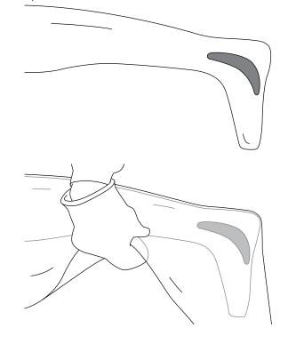
Care should be taken that the polypropylene is sufficiently hot and the trapped air is evacuated fast enough to ensure that the carbon composite inserts are properly encapsulated by the plastic. Proper results have been achieved when the plastic surrounding the inserts presents a well sculptured appearance.
